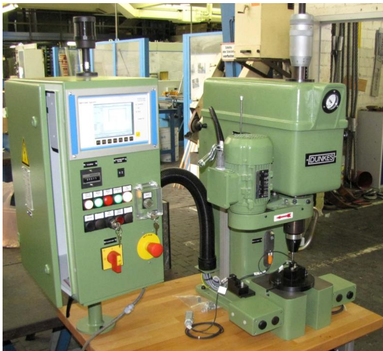
Picture 1 : Example of equipment with a force/path measuring device on a standard riveting machine, model DN 2
